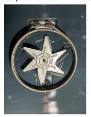
Remove the 2 T-20 Torx screws to the convection element. To remove the motor, remove the 3 T-20 Torx screws and the fan blade then pull motor from the back of the unit.
