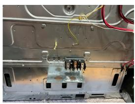
The bake element has 2 hooks on the front, so push the element forward and tilt front of the element upward and pull the element out the rear of the unit. Extra insulation may need to be trimmed when reinstalling the element.
