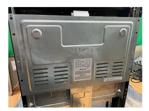
From inside the unit, remove the 4 T-20 Torx screws holding the element in place, and pull unit out from front.
