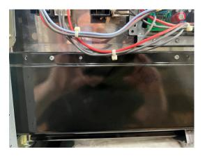
Lift the user interface up and off the back plate and upright stantions. Remove the 4 T-20 Torx to the backsplash and lift off the chassis.
