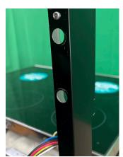
Remove the 4 T-20 Torx screw holding on the upright covers.
