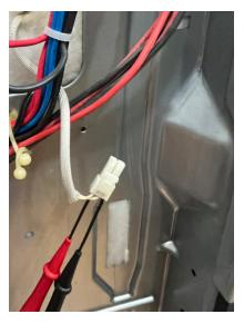
From inside the unit, remove the 2 T-20 Torx screws and remove the temperature probe.
