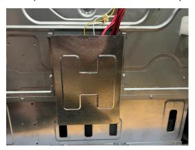
Disconnect the wires to the element and the 3 T-20 Torx fpr the shield for the bake element and the 2 T-20 Torx for the element.
