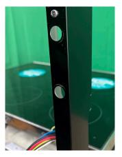
Remove the 4 T-20 Torx securing the cooktop to the rear braket.
