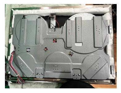
Remove the 8 T-20 Torx screw holding on the upright burner assembly heat shield to the glass top. Disconnect the hot surface indication light wires
