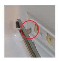
3. Place interlocked shim on both sides of the rear screw hole of the glide (if interlocked shim is too large you can unlock and use single side). You should have 2 shims on each glide.
