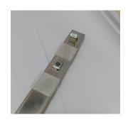
4. Reattach glide rail making sure the shims properly fill the gap as shown below. Once glide rails are reinstalled, install crisper drawer.
